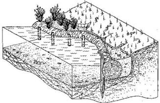
6. An alternative to rock is the use of a coir fiber roll.\* It is pinned securely to the soil, at or above the water line. If this is used, the erosion occurring can be allowed to selfstabilize as the fiber roll will catch the sediment and begin to establish a new stable slope. Native vegetation can be added to the base of the slope as the new slope establishes itself.
